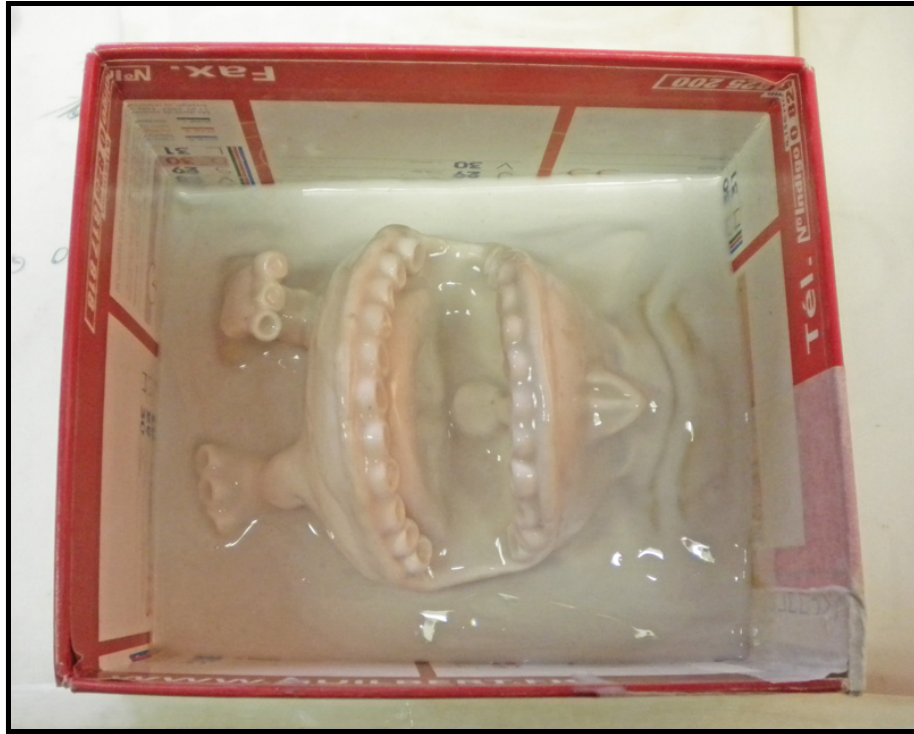
Imprints of the parts in the white silicone mold cast in a cardboard box
