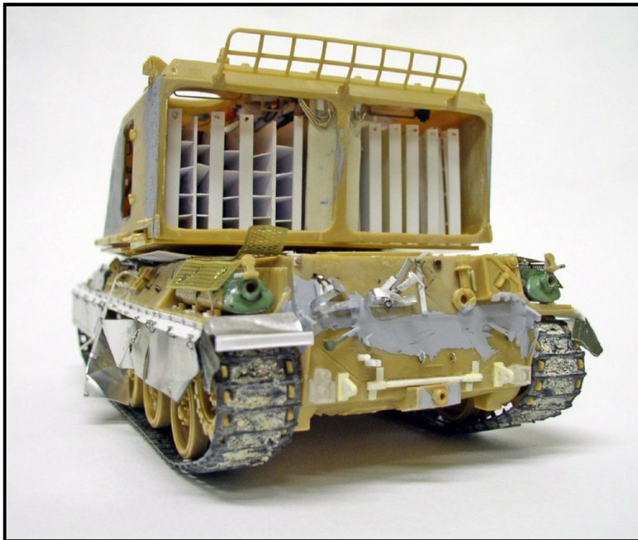
The uneven alignment of the "shelves" is intentional, as they are movable...
